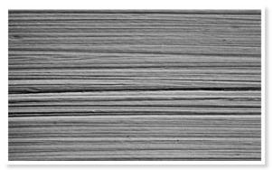
Clearly surfaces on this nature have the propensity to trap dirt and contaminants whilst their roughness hinders proper cleaning as well as an even formation of the passive layer. Equally, it can be seen that orientation of the finish in service will also have an effect with vertical orientation of the 'scratches' being preferred.
