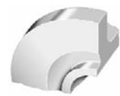
Type H 'O' Ring groove
