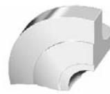
Type G 'O' Ring recess
