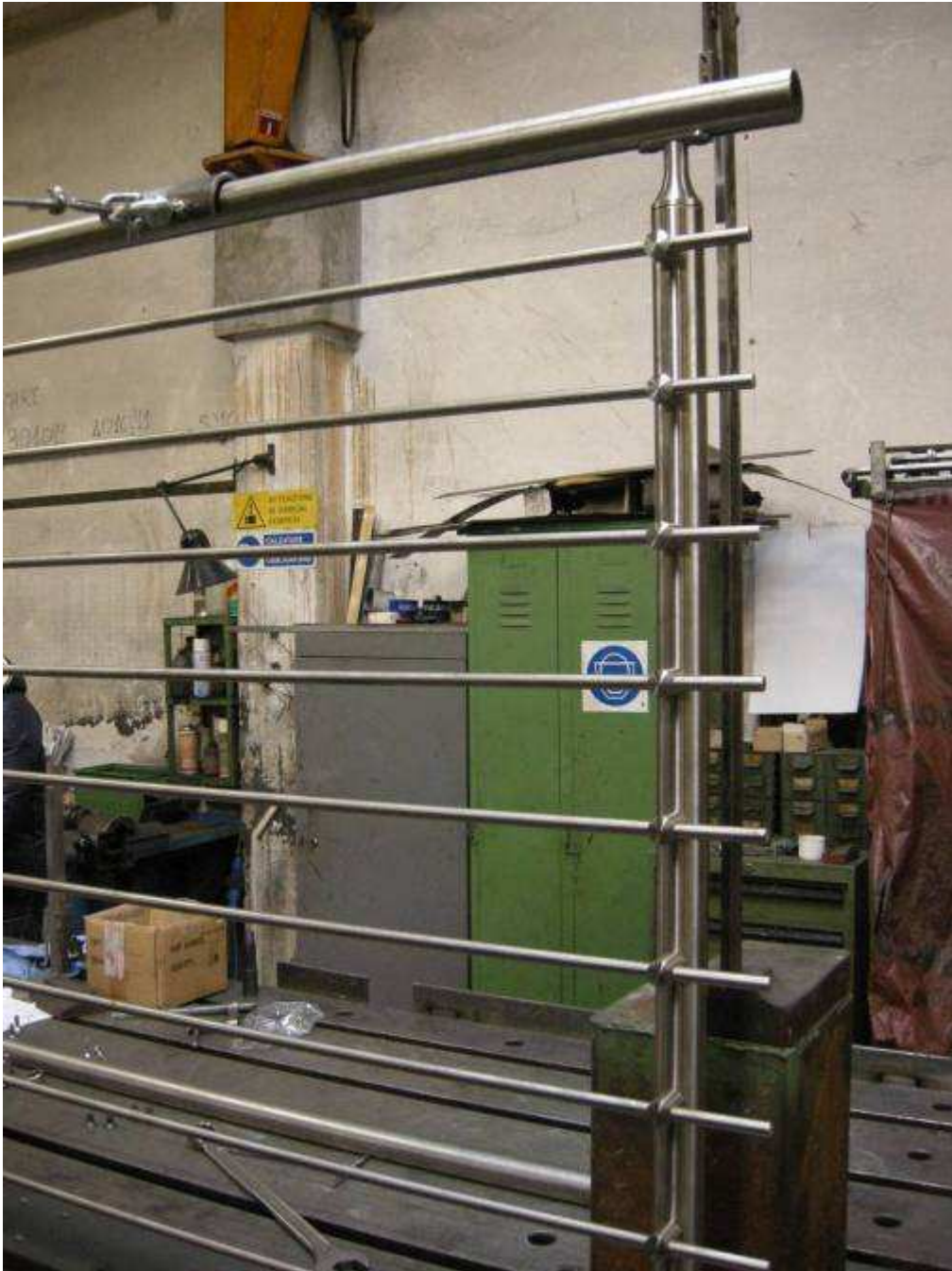
Fig#7_Kit 1 – 1.5 kN during test.
