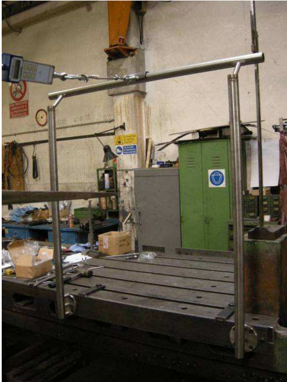
Fig#6_Kit 2 – 3 kN extra strong during test.
