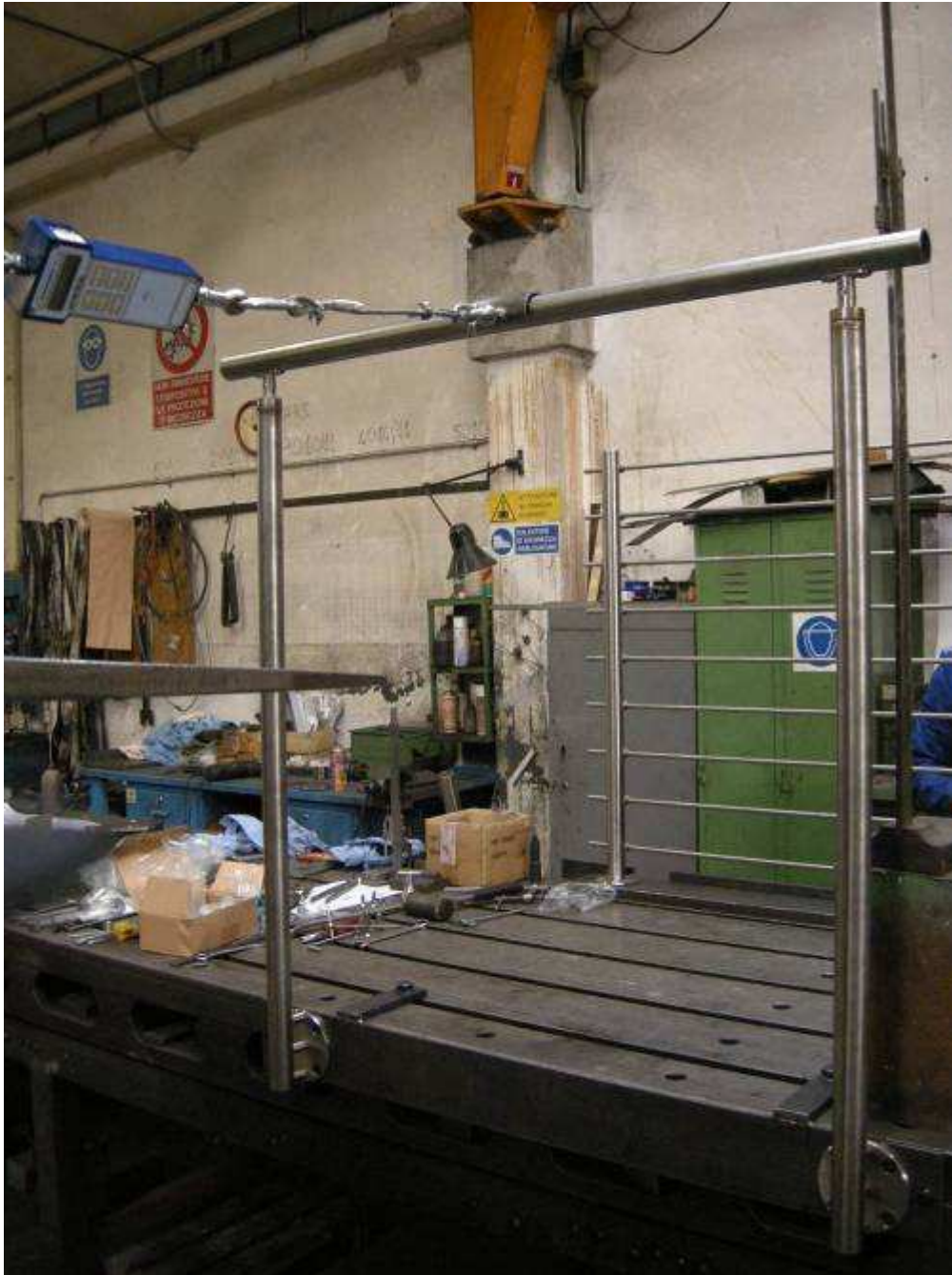
Fig#5_Kit 3- 3 kN extra strong during test.
