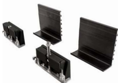
Glass fixing kit - use 1 kit (4 blocks) for each metre of profile. For higher loadings (1.5kN) - use kit containing 6 blocks per metre.
